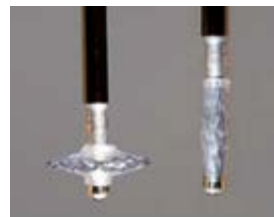
Fig. 4 – Deployed & Collapsed Disc
